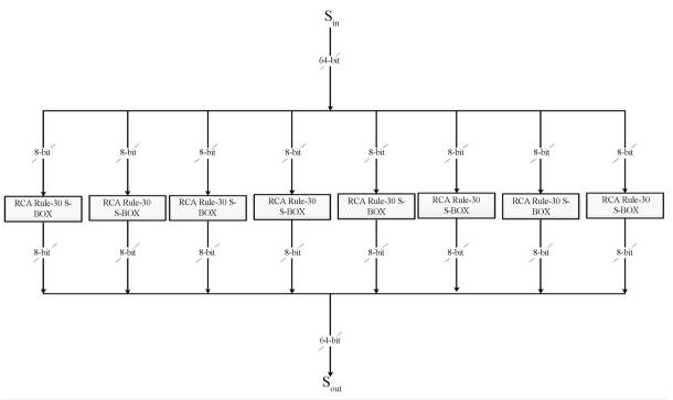
Figure 2. Internal structure of RCA rule-30 based S-BOX.
