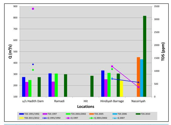
Figure 7. Variation of Discharges (Q) and Total Dissolved Solids (TDS) along Euphrates River inside Iraq.
