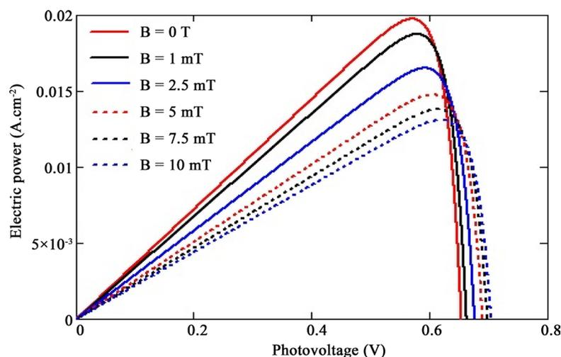
**Figure 3.** Electric power-photovoltage curves for various magnetic field intensity ( $L = 0.02$  cm;  $H = 0.03$  cm;  $D = 26$  cm<sup>2</sup>/s;  $\mu_n = 1000$  cm<sup>2</sup>/V.s).
