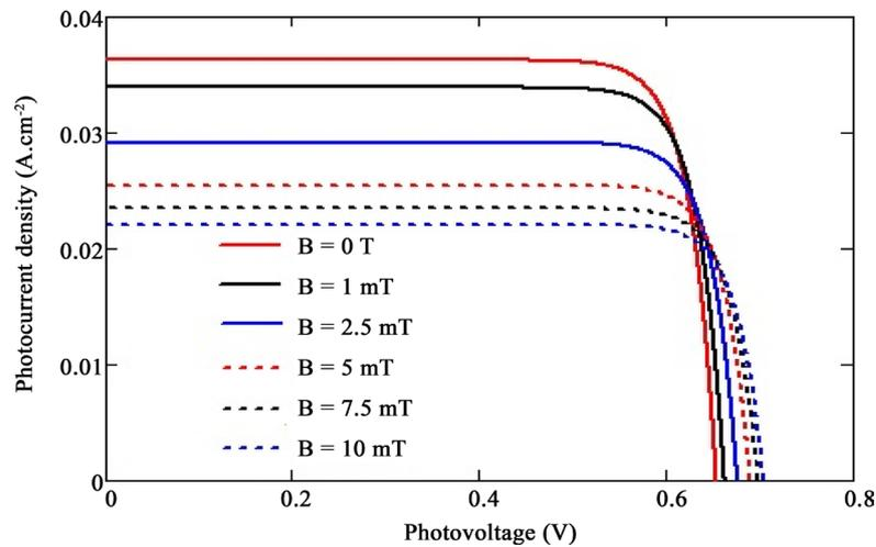
**Figure 2.** Photocurrent density-photovoltage curves for various magnetic field intensity ( $L = 0.02$  cm;  $H = 0.03$  cm;  $D = 26$  cm<sup>2</sup>/s;  $\mu_n = 1000$  cm<sup>2</sup>/V.s).
