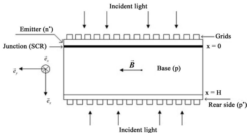
Figure 1. Bifacial silicon solar cell illuminated by multispectral light and under magnetic field influence.
