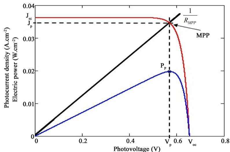
**Figure 4.** Electrical parameters determination using  $J_{ph}$ - $V_{ph}$  and  $P$ - $V_{ph}$  characteristics.
