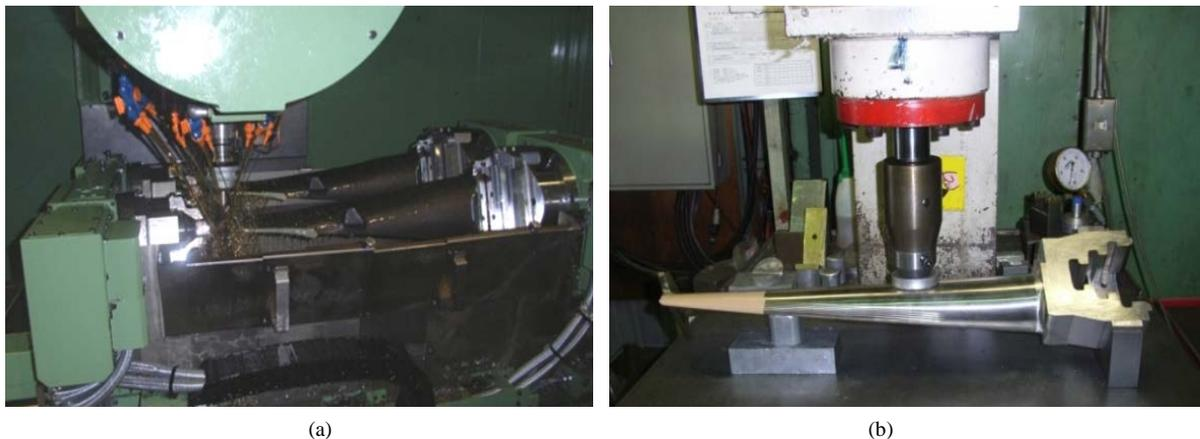
**Figure 1.** Cutting by simultaneous NC milling (a) and the stage of correcting deformation with a press (b).
