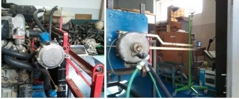
**Figure 5.** Test setup with the loading unit on right and hydrogen supply system on left.
