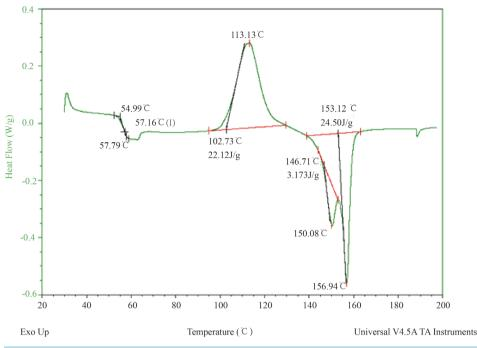
Figure 3. DSC thermograms of sample B3 (5 wt% reinforcement).
