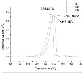
Figure 2. DTG curves for samples B1, B2 and B3.
