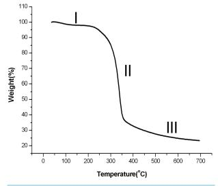
Figure 1. Thermal degradation curve of treated LC fiber (sample C).
