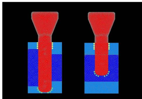
**Figure 4.** Points for measurement of von Mises equivalent stress. The implant collar is indicated in yellow and the implant apex in green. (left) Fibular model. (right) Transplantation model.
