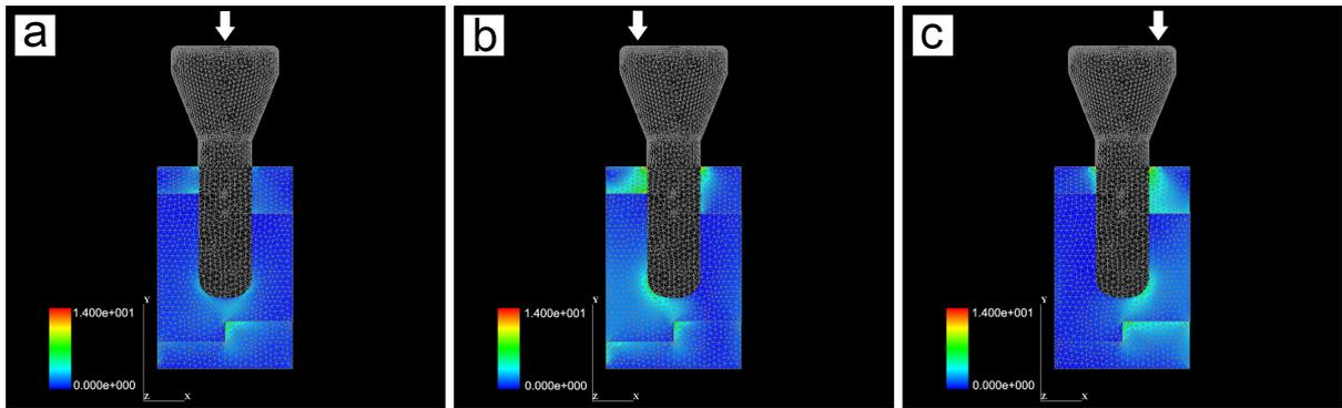
**Figures 8.** In TMM, the mesiodistal cross sections of von Mises equivalent stress contour patterns with a color bar ranging from 0.000e+000 to 1.400e+001 MPa (N/mm<sup>2</sup>). (a) Center loading. (b) Mesial loading. (c) Distal loading.
