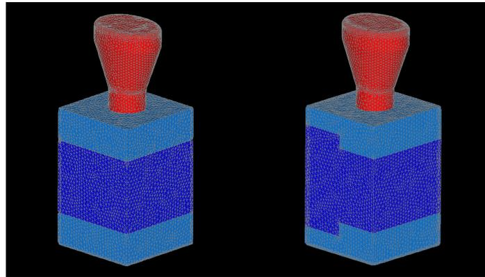
**Figure 1.** (Left) Fibular model with an implant. (Right) Transplantation model with an implant. The size of both models were width 10 mm × depth 10 mm × high 15 mm.
