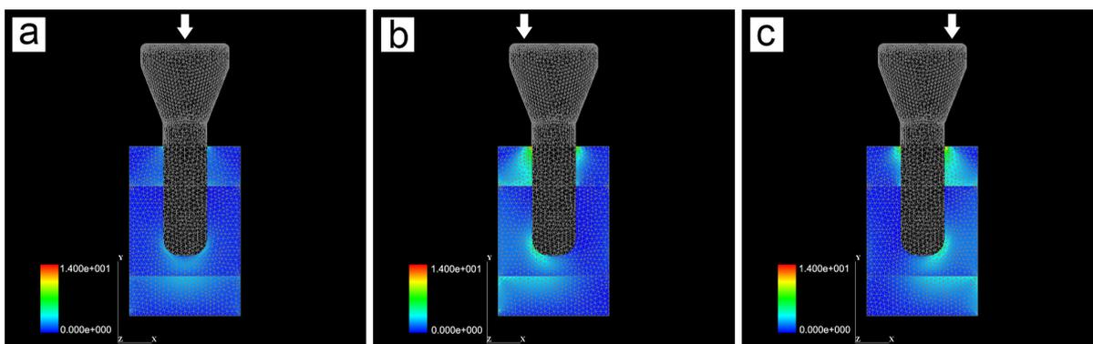
Figure 6. In FMM, the mesiodistal cross-sections of von Mises equivalent stress contour patterns with a color bar ranging from 0.000e+000 to 1.4000e+001 MPa (N/mm<sup>2</sup>). (a) Center loading. (b) Mesial loading. (c) Distal loading.
