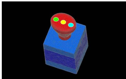
**Figure 3.** The force was set at 2 mm and loading positions set at the center (yellow), mesial (green), and distal (blue) points on the upper surface of the prosthesis, respectively.
