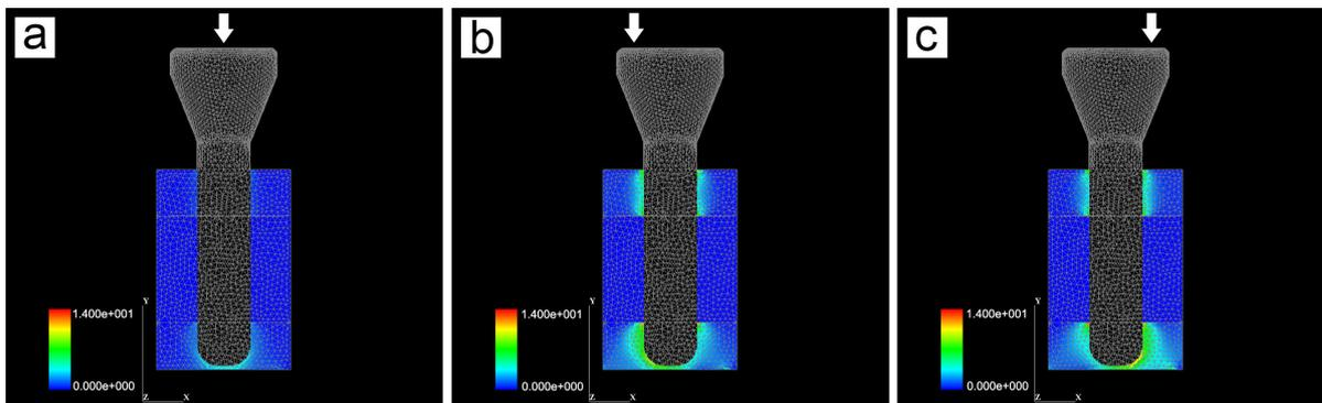
Figure 5. In FMB, the mesiodistal cross sections of von Mises equivalent stress contour patterns with a color bar ranging from 0.000e+000 to 1.4000e+001 MPa (N/mm<sup>2</sup>). (a) Center loading. (b) Mesial loading. (c) Distal loading.
