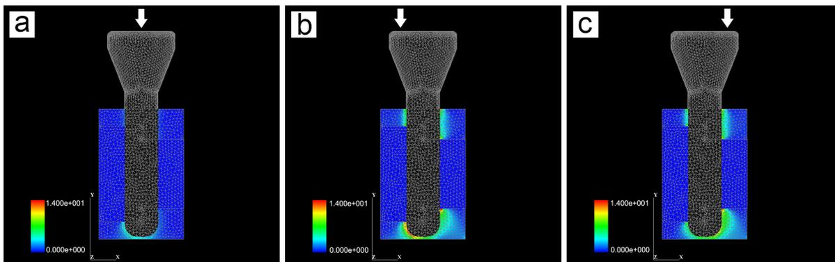
Figure 7. In TMB, the mesiodistal cross-sections of von Mises equivalent stress contour patterns with a color bar ranging from 0.000e+000 to 1.4000e+001 MPa (N/mm<sup>2</sup>). (a) Center loading. (b) Mesial loading. (c) Distal loading.
