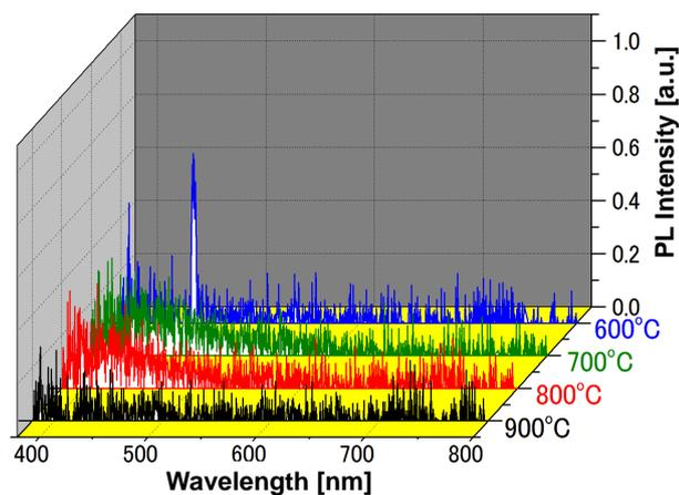
**Figure 3.** PL spectra of CuO-Ta<sub>2</sub>O<sub>5</sub> films annealed at 600°C, 700°C, 800°C, and 900°C.
