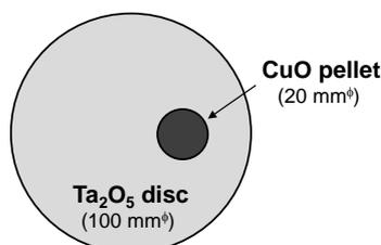
**Figure 1.** Schematic top view of the sputtering target for co-sputtering of a CuO pellet and a Ta<sub>2</sub>O<sub>5</sub> disc.
