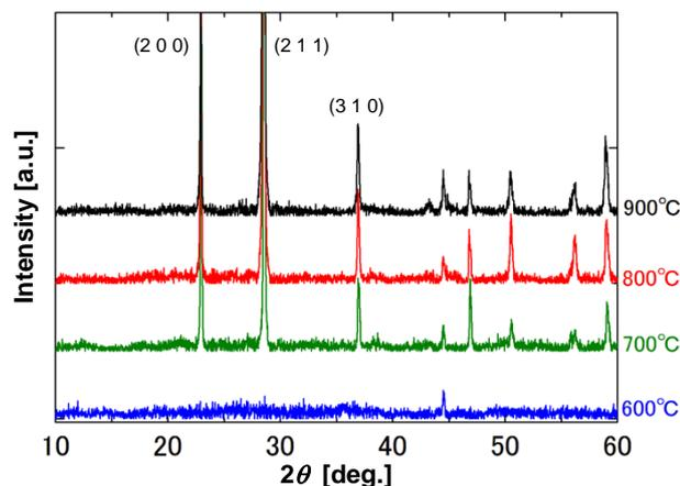
**Figure 2.** XRD patterns of CuO-Ta<sub>2</sub>O<sub>5</sub> films annealed at 600°C, 700°C, 800°C, and 900°C.
