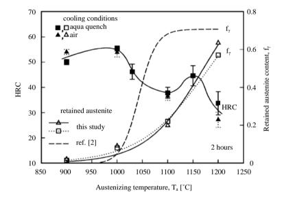
Figure 4. An obvious drop of hardness of X30CrMoN15-1 after the austenitizing temperature exceeds 1000°C.
