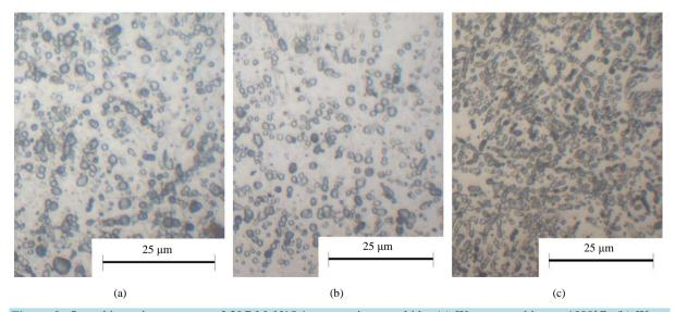
Figure 2. Quenching microstructure of 30CrMoN15-1: martensite + carbide. (a) Water quenching at  $1000^{\circ}$ C; (b) Water quenching at  $900^{\circ}$ C; (c) Air quenching at  $1000^{\circ}$ C.
