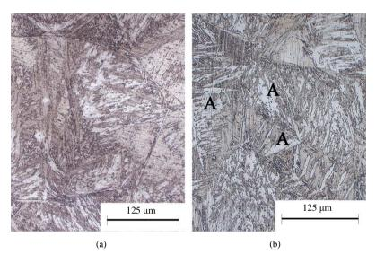
**Figure 1.** Quenching microstructure of 30CrMoN15-1: martensite + carbide + retained austenite. (a) Quenching in ethylene glycol at 1200°C; (b) Quenching in air at 1200°C.
