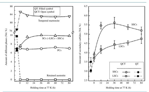
Figure 9. Deep cryogenic treatment influences amount of the small second carbide and large second carbide.
