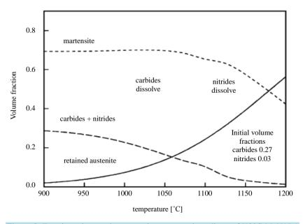
Figure 8. Function relevance between microstructure ingredients of X30CrMoN15-1 and quenching temperatures with deep cryogenic treatment following after quenching.
