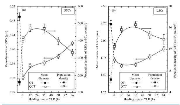
Figure 10. Deep cryogenic treatment influences the sizes and distribution density of the small second carbide and large second carbide.
