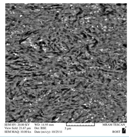
Figure 11. The finer spheric second carbide particles observed in deep cryogenic treatment of 1.2542.
