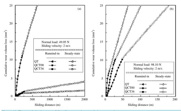
Figure 12. The correlation between sliding distance and accumulative wear volume.
