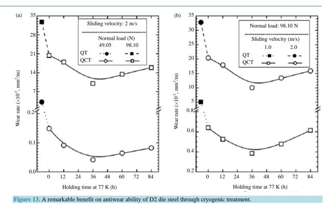
A remarkable benefit on antiwear ability of D2 die steel can be achieved through cryogenic treatment as showed in Figure 13. In case of FN = 98.1 N, Vs = 1 m/s and FN = 49.05 N, Vs = 2 m/s, the antiwear ability rises as high as 13.2 times and 76.2 times respectively if there is a cryogenic treatment compared to there isn't.
