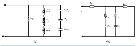
Figure 3. (a) Equivalent circuit of RMSA due to notch effect; (b) Equivalent circuit of H-shaped fed patch.
