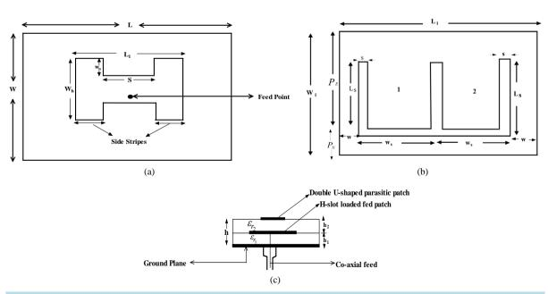
Figure 1. Configuration of stacked patch antenna. (a) H-slot loaded fed patch; (b) Double U-shaped slots loaded parasitic patch; (c) Side view of the proposed antenna.
