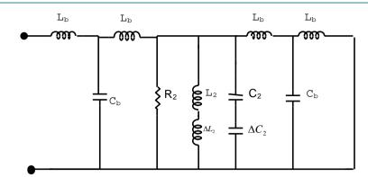
Figure 4. Equivalent circuit of U-slot loaded patch.
