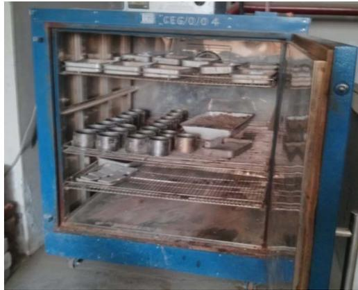
**Figure 5.** Pre heating of moulds.
