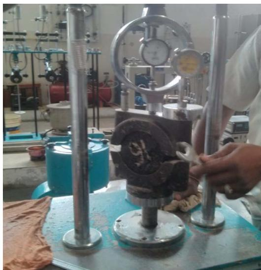
Figure 9. Performing marshal stability test.
