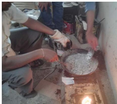
**Figure 4.** Adding shredded plastic to aggregates.
