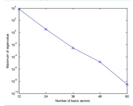
Figure 4. Maximum norm of projection error changing with the increasing of number of basis vectors.
