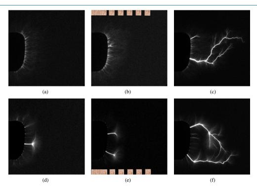
**Figure 7.** Discharge images, taken sequentially in the burst. Top row ((a)-(c)) positive polarity; bottom row ((d)-(f)) negative polarity. The pulse pair number is #1 ((a) and (d)), #2 ((b) and (e)), and #8 ((c) and (f)). The HV electrode and CS positions are indicated by insertion in (b) and (e) images.
