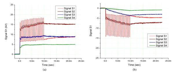
**Figure 3.** Surface charge sensors typical traces. S1-S4—sensor numbers from closest to exposed electrode to the furthest away. (a) Positive polarity; (b) Negative polarity.
