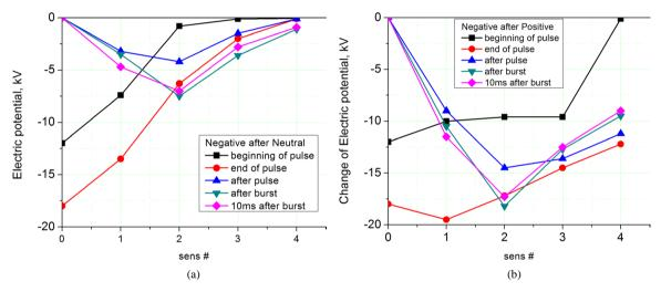
**Figure 5.** Electric potential distribution over the surface at and after the negative pulses. (a) No discharge contraction; (b) Discharge contraction observed.
