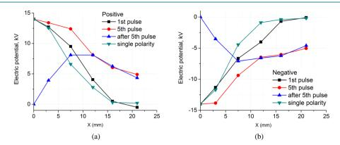
**Figure 8.** Typical distribution of the electric potential over the surface for the  $1^{st}$  pulse in the burst, at the 5<sup>th</sup> pulse, after the 5<sup>th</sup> pulse, and for a single polarity at the 8<sup>th</sup> pulse. (a) Positive polarity; (b) Negative polarity.
