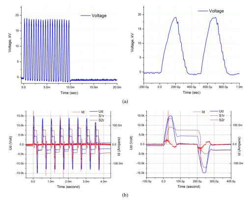
**Figure 2.** Typical waveforms in a burst mode of single (a) and alternating (b) polarities. Discharge voltage, Ud; discharge current Id; data from the first sensor, S1; and data from the second sensor, S2.
