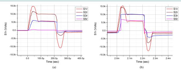
**Figure 6.** The surface electric potential dynamics depending on the pulse number, detail view. (a) The first positive and negative pulses; (b) The 8<sup>th</sup> positive and negative pulses.
