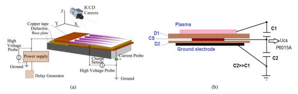
Figure 1. Experimental test cell layout (a); Scheme of the charge sensor assembly (b).
