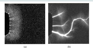
**Figure 4.** ISSD camera images of the SDBD in diffusive (a) and contraction (b) mode. Negative polarity, first pulse in the burst.
