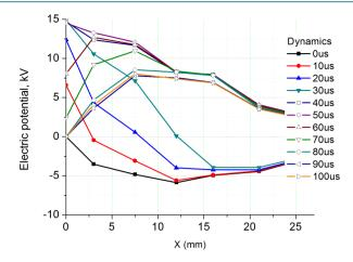
**Figure 9.** Dynamics of the X-distribution of the surface potential during and after the  $\tau = 50 \ \mu s$  positive pulse following the negative pulse,  $U_{max} = 15 \ kV$ .
