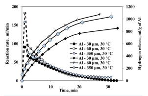
**Figure 2.** Reaction rate (dotted line) and hydrogen evolution rate (solid line) of the activated aluminum mixtures with water at 30°C, Al-85% and Galinstan eutectics 15% by mass (Ga-In-Sn-Zn = 60-25-10-5).
