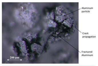
Figure 1. Crack formation on the activated aluminum particles at ~30°C.
