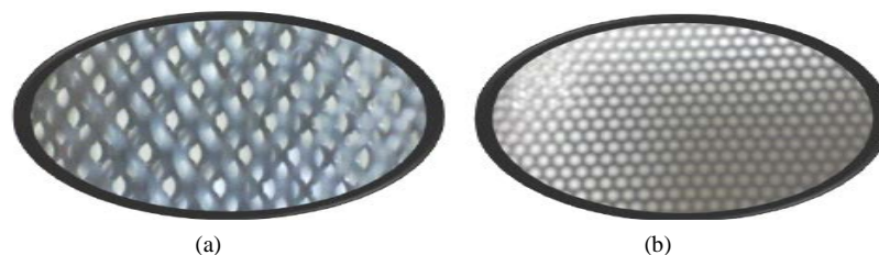
Figure 2. (a) and (b): Aluminum Meshes with different number of holes per inch, (a) Al mesh of 3 mm width of hole and 8 holes per inch; (b) Al other mesh of 0.3 mm width of hole and 20 holes per inch.
