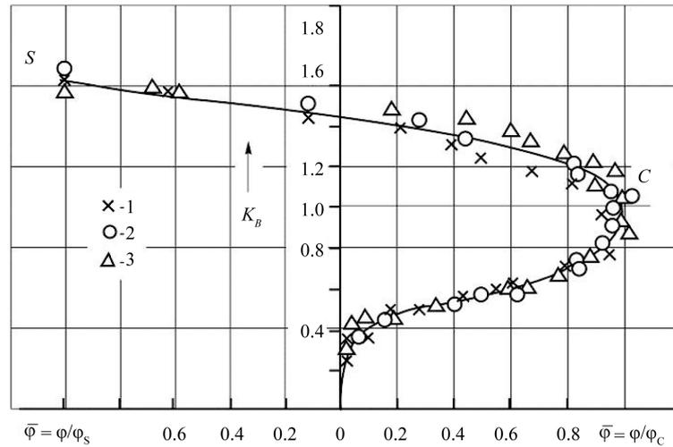
**Figure 3.** Generalized  $D$ -diagrams of the cyclic elasto-plastic fracture for the carbonic steel constructed by the results of tests of compact samples of 10 (1), 20 (2) and 40 (3) mm thickness.
