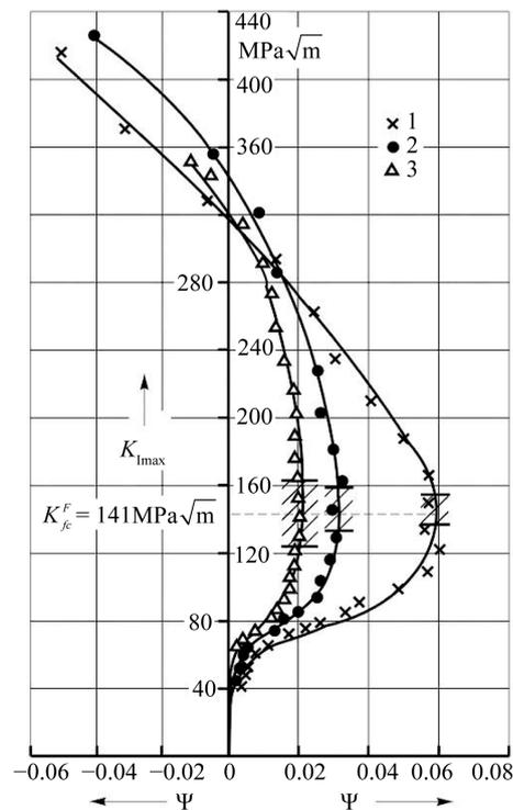
**Figure 2.**  $D$ -diagrams of the cyclic elasto-plastic fracture for the carbonic steel constructed by the results of tests of compact samples of 10 (1), 20 (2) and 40 (3) mm thickness.
