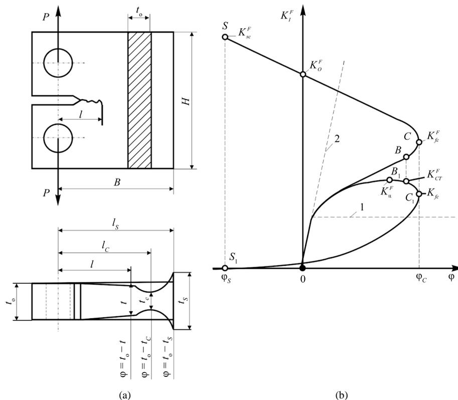
**Figure 1.** Schemes: test of the compact specimen and measurement of the thickness reduction (a); cyclic elasto-plastic fracture diagram for a specimen with a crack (b).
