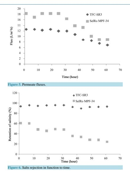
for SelRo MPF-34 the rejection rate is constant during 7 hour, beyond the rejection rate decreases gradually till 27% at 61 hour functioning.
