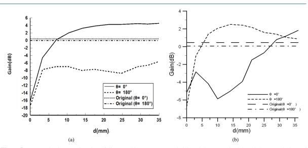
Figure 5. Measured gains as a function of distance d between (a) metal slab and (b) magnetic slab and the ground plane of monopole antenna.
