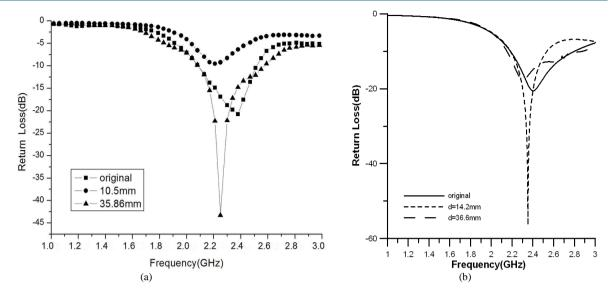
Figure 3. The return loss of (a) metal slab and (b) magnetic slab of the monopole antenna as a function of the spacing.
