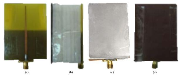
Figure 2. The (a) top, (b) side, (c) metal slab with bottom and (d) magnetic slab with bottom view of antenna.
