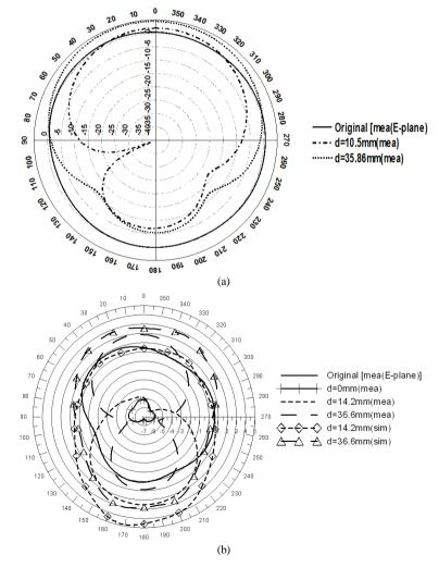
Figure 4. Simulated and measured patterns as a function of distance d between the (a) metal slab and (b) magnetic slab and the ground plane of monopole antenna.
