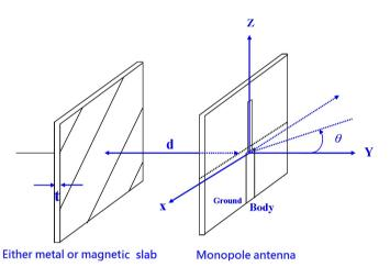
Figure 1. Schematic diagram of monopole antenna and either metal or magnetic slab.
