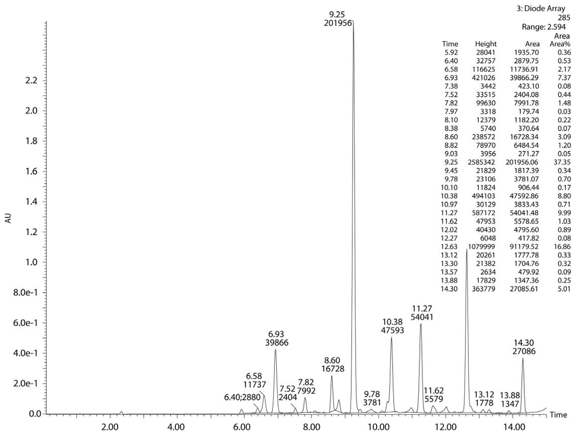
Figure 5. Base degradation chromatogram of Lansoprazole.
