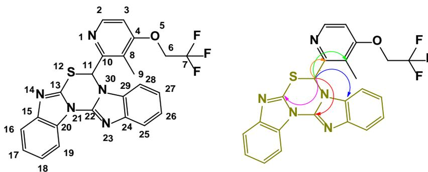
Figure 8. Numbering scheme and HMBC correlation structures of base degradation product.
