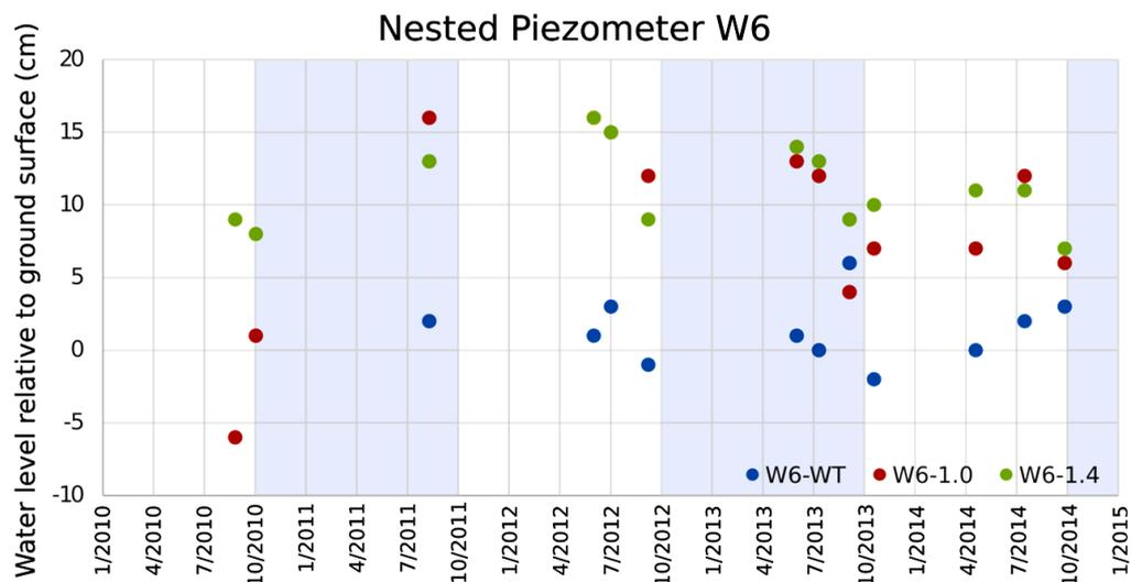
**Figure 12.** Water levels measured in the W6 piezometer cluster at Wilshire fen. Depth of the W6-WT piezometer was measured at 102 cm on 2-June-2012 (reported at 105 cm [4]). The piezometer was screened to 95 cm in peat. The W6-1.0 piezometers was measured at 104 cm bgs on 2-June-2012 (reported depth of 112 cm [4]). The W6-1.4 piezometer was measured at 144 cm bgs on 2-June-2012 (reported depth of 141 cm [4]).
