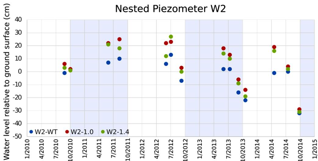
**Figure 10.** Water levels measured in the W2 piezometer cluster at Wilshire fen. The patterns observed in the W2 piezometer cluster are similar to those observed in the W1 and W5 clusters. The depth of the W2-WT piezometer was measured at 105 cm bgs on 2-June-2012 and had 95 cm of screen in peat. The depth of W2-1.0, an open-ended piezometer, was measured at 86 cm bgs on 2-June-2012. The depth of W2-1.4, an open-ended piezometer, was measured at 144 cm bgs on 2-June-2012.
