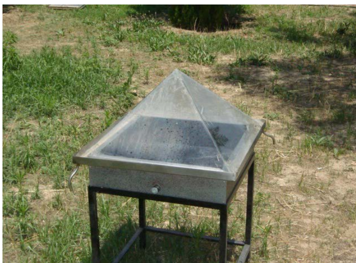
Figure 3. The fabricated solar still being tested in outdoor conditions.
