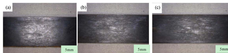
Figure 6. Photographs of surface of specimens (fiber 100%). a) 160°C; b) 180°C and c) 200°C.
