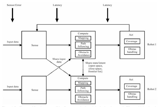
Figure 1. Intelligent mobile robots are traditionally structured using a behavior-based approach. When multiple robots interact, new sources of discrepancy, such as message production and processing, can cause simulations to vary from experiments.
