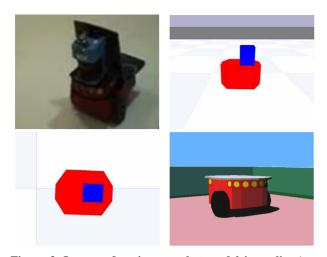
Figure 3. Images of a pioneer robot model in reality (top left), stage (top right), stage from top view (bottom left), and webots (bottom right).
