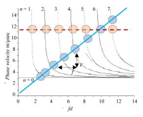
Figure 4. Dispersion curves and the activation lines of the guided waves.
