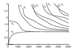
Figure 3. Dispersion curves of the phase velocity in plate structure;  $S_n$  symmetric Lamb waves;  $A_n$  asymmetric Lamb waves.
