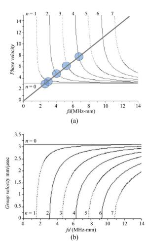
Figure 5. Shear waves dispersion curves for stainless steel plate with thickness 5.89 mm. (a) phase velocity (mm/µsec); (b) group velocity (mm/µsec).
