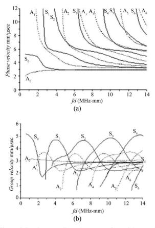
Figure 6. Lamb waves dispersion curves for stainless steel plate with thickness 5.89 mm. (a) phase velocity (mm/µsec); (b) group velocity (mm/µsec).
