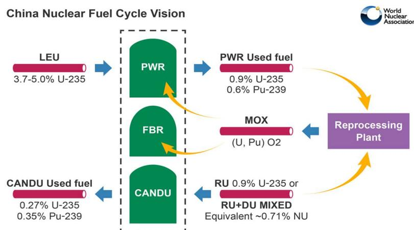
**Figure 3.** Illustration of Chinese nuclear fuel cycle [4].
