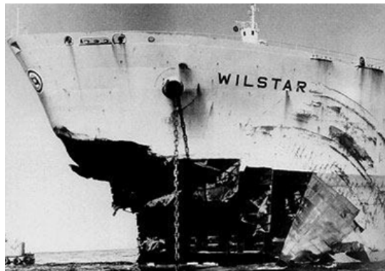
Figure 5. The WILSTAR Norwegian cargo boat hit by a rogue waves [49].
