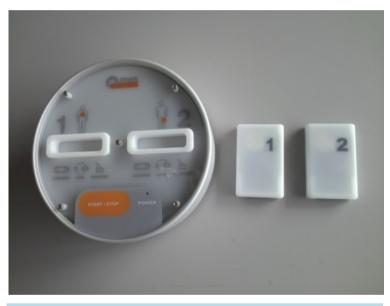
Figure 1. The activity monitoring and evaluation system (A-MES) (right: sensors; left: station).
