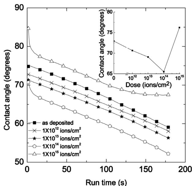
**Figure 4.** Dynamic contact angle for different Argon ion irradiation. Inset figure was plotted for the change of contact angle as a function of ion doses where the contact angles were taken at 30 sec run time.
