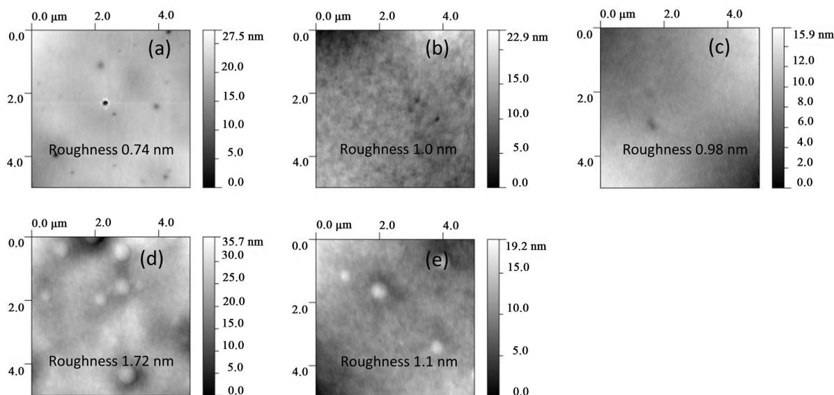
**Figure 2.** Tapping-mode atomic force microscopy 2-D images of (a) as deposited PLGA and Argon ion irradiated PLGA with doses (b)  $1 \times 10^{12}$  ions/cm<sup>2</sup>, (c)  $1 \times 10^{13}$  ions/cm<sup>2</sup>, (d)  $1 \times 10^{14}$  ions/cm<sup>2</sup>, and (e)  $1 \times 10^{15}$  ions/cm<sup>2</sup>.
