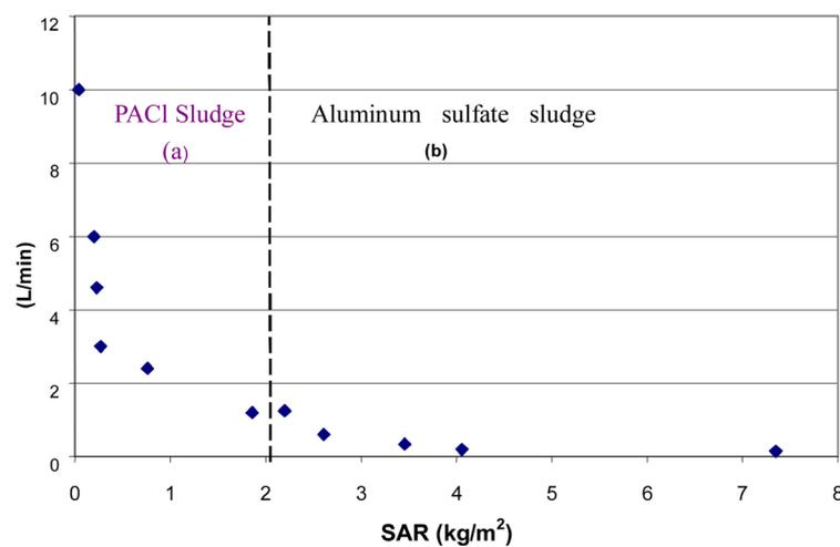
Figure 5. Relation between initial drainage flow of free water (L/min) and the values of Surface Application Rate—SAR (kg/m<sup>2</sup>) for tests conducted with a sample of PACl sludge (a) and  $Al_2(SO_4)_3$  sludge (b).
