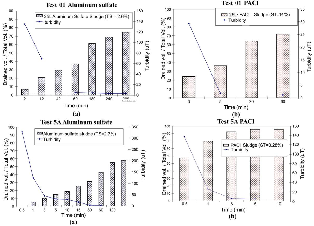
Figure 6. Variation in the values of cumulative volume of drained free water (%) and turbidity during the Drainage Phase, for samples of  $Al_2(SO_4)_3$  (a) and PACl (b).
