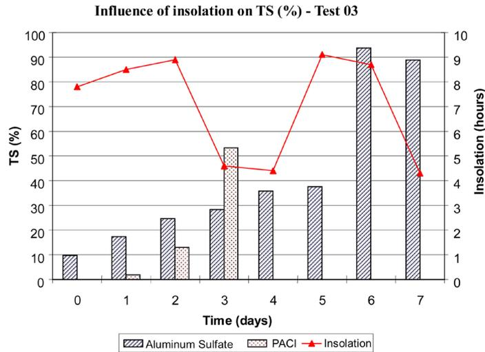
Figure 7. Variation of insolation and total solids content (% TS) for one of the Drainage Bed dewatering tests (Drying Phase).
