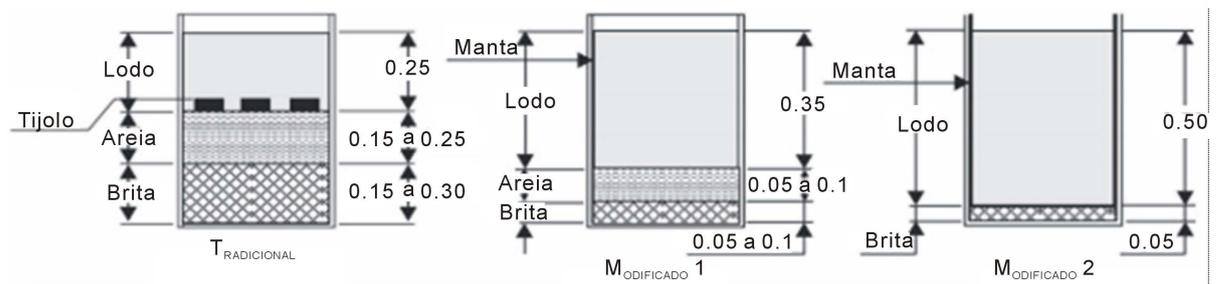
**Figure 1.** Illustrative schemes of traditional and modified systems 1 and 2 (Drainage Bed) as proposed by Cordeiro (1993 and 2000) [9] and [10].
