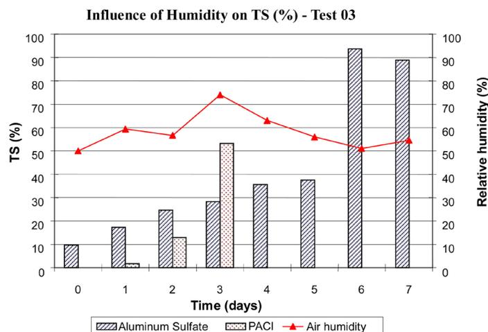
**Figure 8.** Variation of humidity and total solids content (%TS) for one of the Drainage Bed dewatering tests (Drying Phase).
