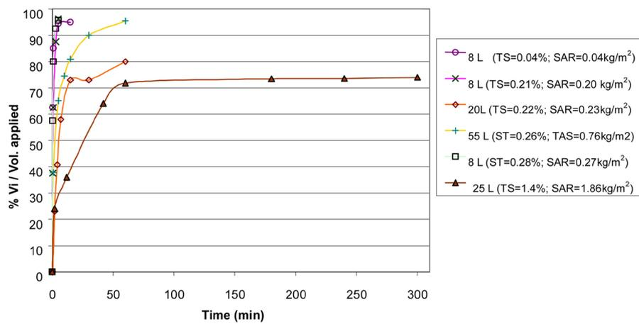
Figure 4. Cumulative volume of drained free water in dewatering tests with PACl sludge samples.
