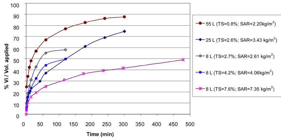
Figure 3. Cumulative volume of drained free water in dewatering tests with  $Al_2(SO_4)_3$  sludge samples.
