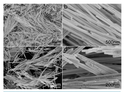
Figure 3. SEM images of the as-synthesized products with the molar ratio of GeO<sub>2</sub> to CdO of (a) 2:1 and (b) 1:1. CTAB was added as surfactant.
