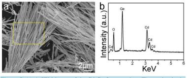
**Figure 5.** (a) A SEM image of the  $Cd_2Ge_2O_6$  nanowires. The section in the yellow rectangle was taken for data collection; (b) Energy dispersion X-ray spectrum of the as-prepared product.
