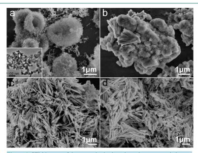
Figure 1. SEM images of the as-synthesized products that were carried out at (a)  $120^{\circ}$ C; (b)  $140^{\circ}$ C; (c)  $160^{\circ}$ C and (d)  $180^{\circ}$ C for 24 h. The inset is the high magnified TEM image of the nanoparticles.
