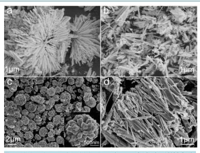
**Figure 2.** SEM images of the  $Cd_2Ge_2O_6$  products synthesized at 180°C for 24 h with (a) EDA; (b) PVP; (c) SDBS and (d) CTAB added as surfactant.
