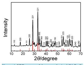
**Figure 4.** XRD pattern of the as-synthesized Cd<sub>2</sub>Ge<sub>2</sub>O<sub>6</sub> product prepared using GeO<sub>2</sub> and CdO as the precursors.
