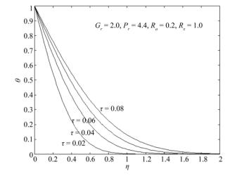
Figure 6. Temperature distributions  $\theta$  with  $P_r = 4.4$ ,  $R_a = 0.2$ ,  $R_x = 1.0$ .
