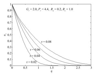
Figure 2. Velocity distributions  $u_1$  with  $G_r = 2.0$ ,  $P_r = 4.4$ ,  $R_a = 0.2$ ,  $R_x = 1.0$ .
