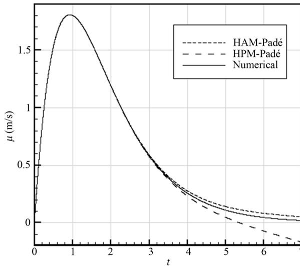
**Figure 2.** The velocity in  $r$  direction for water with  $r = 0.01$ ,  $\omega = 1000$  rad/s,  $\nu = 1.519 \times 10^{-6}$  (m<sup>2</sup>/s),  $\rho = 1000$  (kg/m<sup>3</sup>).
