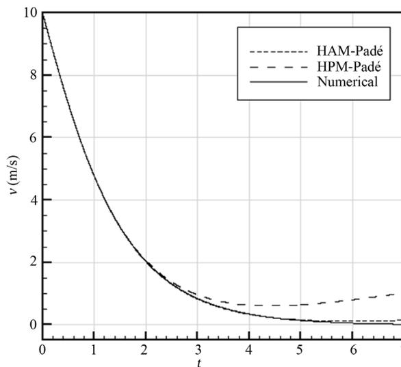
**Figure 3.** The velocity in  $\theta$  direction for water with  $r = 0.01$ ,  $\omega = 1000$  rad/s,  $\nu = 1.519 \times 10^{-6}$  (m<sup>2</sup>/s),  $\rho = 1000$  (kg/m<sup>3</sup>).
