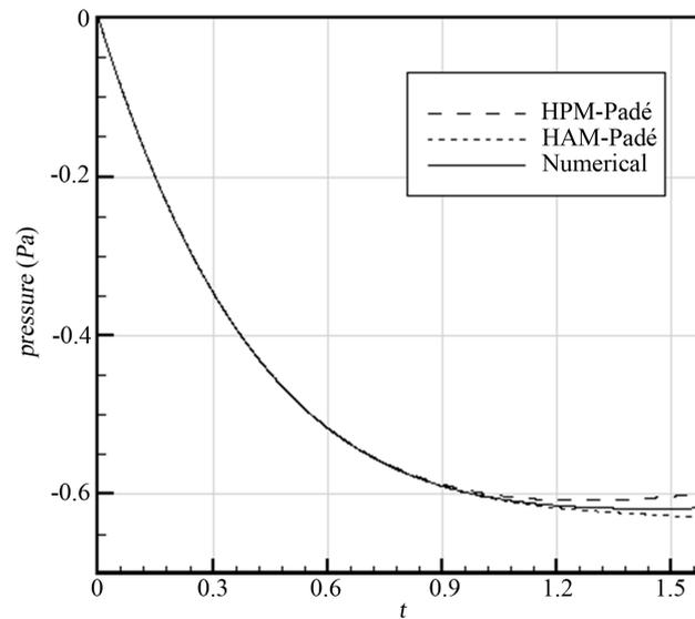
**Figure 5.** The pressure distribution in the  $z$  direction for water with  $r = 0.01$ ,  $\omega = 1000$  rad/s,  $\nu = 1.519 \times 10^{-6}$  (m<sup>2</sup>/s),  $\rho = 1000$  (kg/m<sup>3</sup>).
