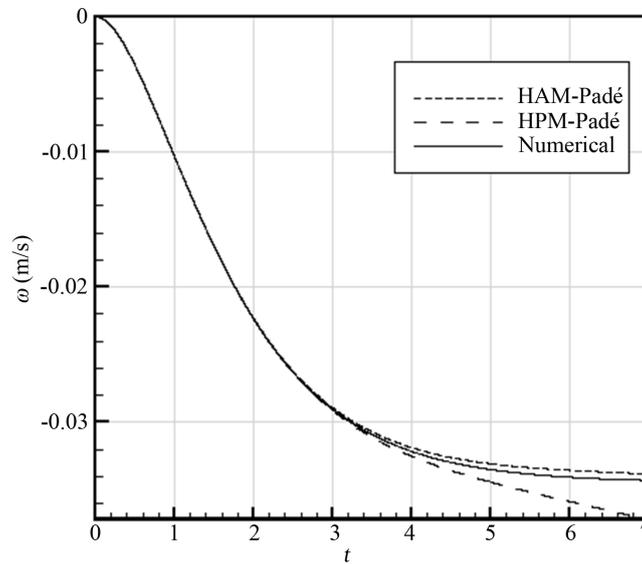
**Figure 4.** The velocity in  $z$  direction for water with  $r = 0.01$ ,  $\omega = 1000$  rad/s,  $\nu = 1.519 \times 10^{-6}$  (m<sup>2</sup>/s),  $\rho = 1000$  (kg/m<sup>3</sup>).
