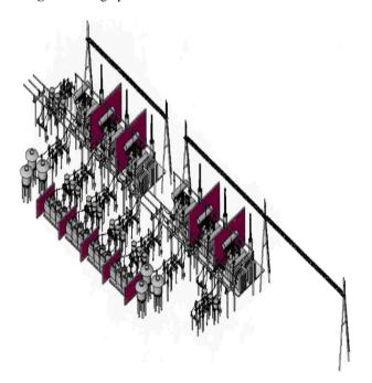
Figure 4. The main transformer and 35 kV power distribution device model.
