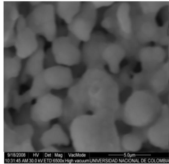
**Figure 3. SEM micrograph for  $\text{Sr}_2\text{GdRuO}_6$  double perovskite obtained from ETD detector (secondary electrons).**
