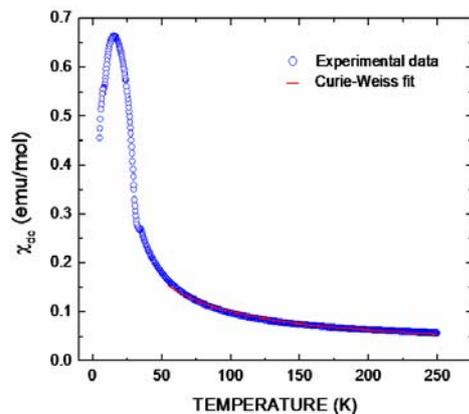
**Figure 4. Measurements of *dc* Susceptibility for  $\text{Sr}_2\text{GdRuO}_6$  on the application of  $H = 0.1 \text{ T}$ . In picture, circles are the experimental data and the line represents the Curie-Weiss fitting.**
