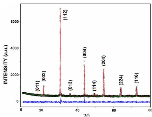
**Figure 1.** XRD pattern for  $\text{Sr}_2\text{GdRuO}_6$  complex perovskite. Symbols correspond to the experimental data and continuous one is the obtained by Rietveld refinement. Bottom curve represents the difference between experimental and calculated patterns.
