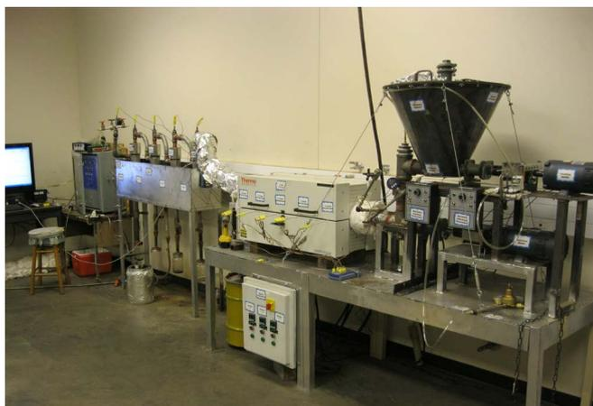
**Figure 1.** The allothermal auger gasification system.
