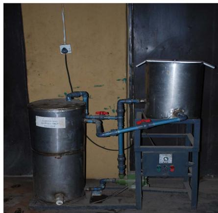
**Figure 3.** The fabricated Jominy end quench machine.
