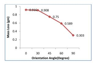
Figure 7. Effect of orientation angle at 5 N
