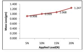
Figure 3. Effect of load at 30° orientation.
