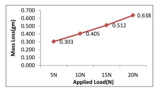
Figure 6. Effect of load at 90° orientation.
