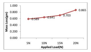
Figure 5. Effect of load at 60° orientation.
