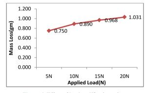
Figure 4. Effect of load at 45° orientation.
