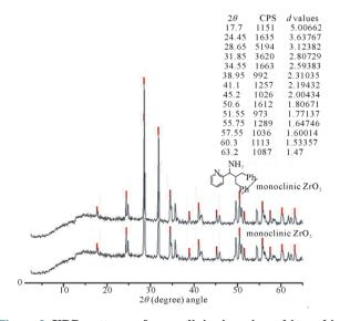
Figure 2. XRD patterns of monoclinic zirconia and immobilized picolylamine on zirconia.
