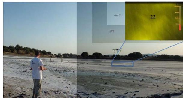
**Figure 6.** The frame composite visible image shows the reconstructed pattern of the second hexacopter flight. Inset shows the frame from the drone-borne thermal camera taken at the same site as field temperature measurements and the temperature measured in the centre of the image.
