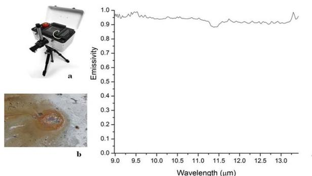
**Figure 5.** (a) μFTIR instrument used to measure emissivity spectrum; (b) Visible image of one of cold pool (20 cm diameter) that was possible to access; (c) Emissivity measured spectrum.
