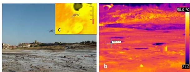
**Figure 4.** (a) Visible image of the area selected for the first flight; (b) thermal image acquired by FLIR camera, the spot is located in correspondence of the same area as seen by the TC 3600 (c).
