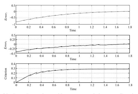
Figure 4. Graphs of the *Error*<sub>1</sub>, *Error*<sub>2</sub>, and exponential mean square cost criterion corresponding to the risk-sensitive optimal filtering equations for satellite monoaxial for  $\varepsilon = 10$ ,  $X_1(0) = 0.115$ ,  $X_2(0) = 0.073$ ,  $Y_1(0) = 2$ ,  $Y_2(0) = 1$ .
