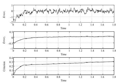
Figure 5. Graphs of the *Error*<sub>1</sub>, *Error*<sub>2</sub>, and exponential mean square cost criterion corresponding to the polynomial filtering equations for satellite monoaxial for  $\varepsilon = 10$ ,  $X_1(0) = 0.115$ ,  $X_2(0) = 0.073$ ,  $Y_1(0) = 2$ ,  $Y_2(0) = 1$ .
