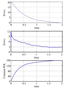
Figure 2. Graphs of the *Error*<sub>1</sub>, *Error*<sub>2</sub>, and exponential mean square cost criterion corresponding to the polynomial filtering equations for a continuous stirred tank reactor for  $\varepsilon = 10$ ,  $X_1(0) = 20$ ,  $X_2(0) = 10$ ,  $Y_1(0) = 2$ ,  $Y_2(0) = 1$ .
