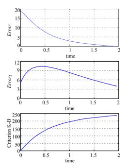
Figure 3. Graphs of the *Error*<sub>1</sub>, *Error*<sub>2</sub>, and exponential mean square cost criterion corresponding to the extended Kalman-Bucy filtering equations for a continuous stirred tank reactor for  $\varepsilon = 10$ ,  $X_1(0) = 20$ ,  $X_2(0) = 10$ ,  $Y_1(0) = 2$ ,  $Y_2(0) = 1$ .
