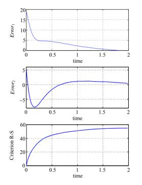
Figure 1. Graphs of the *Error*<sub>1</sub>, *Error*<sub>2</sub>, and exponential mean square cost criterion corresponding to the risk-sensitive optimal filtering equations for a continuous stirred tank reactor for  $\varepsilon = 10$ ,  $X_1(0) = 20$ ,  $X_2(0) = 10$ ,  $Y_1(0) = 2$ ,  $Y_2(0) = 1$ .
