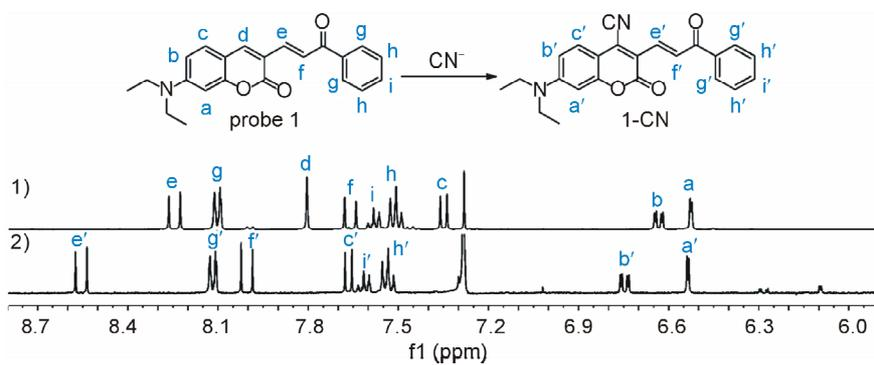
Figure 7. Partial  $^1\text{H}$  NMR (400 MHz) spectra of 1) Probe 1 and 2) the isolated product of Probe 1 +  $\text{CN}^-$ .
