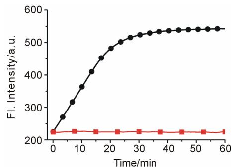
**Figure 5.** Time dependent fluorescence intensity (608 nm) changes of Probe 1 (5  $\mu\text{M}$ ) in the absence (■) or presence (●) of 90  $\mu\text{M}$   $\text{CN}^-$ .
