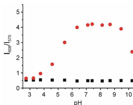
**Figure 6.** The variations of emission ratio ( $I_{608}/I_{570}$ ) of Probe 1 (5  $\mu\text{M}$ ) in the absence (■) or presence (●) of  $\text{CN}^-$  (90  $\mu\text{M}$ ) as a function of pH.
