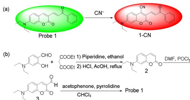
**Scheme 1.** (a) the sensing reaction of Probe 1 with  $\text{CN}^-$ ; (b) the synthetic procedure of Probe 1.
