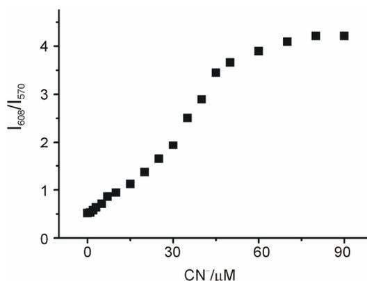
**Figure 2.** Changes in fluorescence emission ratios ( $I_{608}/I_{570}$ ) of Probe **1** (5  $\mu\text{M}$ ) to various amount of  $\text{CN}^-$  (0 to 90  $\mu\text{M}$ ),  $\lambda_{\text{ex}} = 510$  nm.
