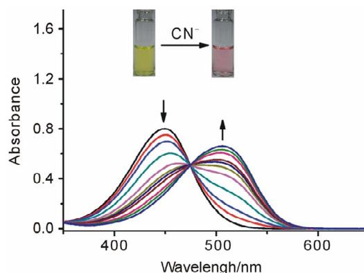
**Figure 3.** Changes in absorption spectra of Probe **1** (5  $\mu\text{M}$ ) with various amount of  $\text{CN}^-$  (0 to 90  $\mu\text{M}$ ), inset: visible color changes of Probe **1** (5  $\mu\text{M}$ ) in the absence and presence of  $\text{CN}^-$  (90  $\mu\text{M}$ ).
