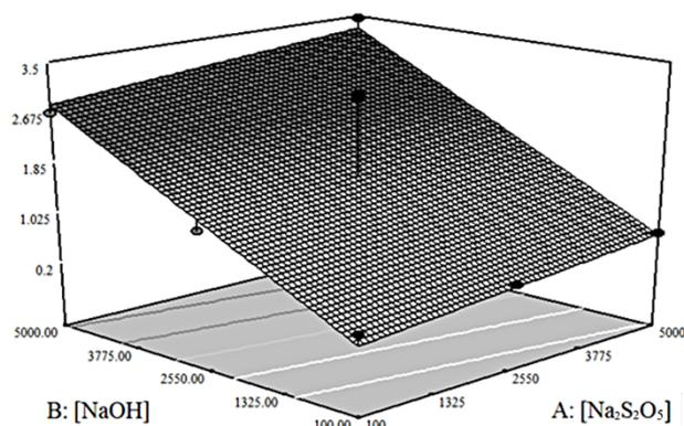
**Figure 4.** 3D surface of ash content.
