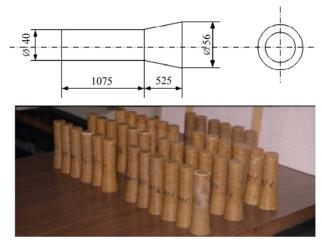
Figure 1. The samples of fatigue experiment.
