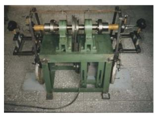
Figure 4. The bending, fatigue experiment device.
