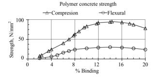
Figure 2. Polymer concrete compressive and flexural strength change.
