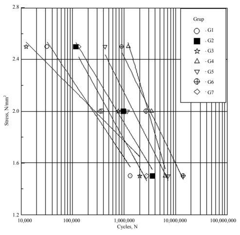
Figure 5. The results of fatigue tests for polymer concrete samples.
