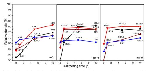
Figure 1. Variation of the relative density of Al<sub>2</sub>(WO<sub>4</sub>)<sub>3</sub> pellets, depending on sintering temperature (800°C, 900°C and 1000°C), sintering time (0, 1, 5 and 10 h) and average particle size in the raw pellets (-n-20 nm,  $-\sqrt{-90}$  nm,  $-\Delta-200$  nm and  $-\bullet->1$  µm). 3.8/3 - 3.8 is the average particle size after appropriate sintering [µm]; 3 is the average ratio between the largest and the smallest particle size.
