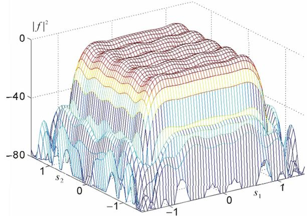
**Figure 23.** The synthesized power DP  $|f|^2$  for  $N_0=1$  at  $c_1 = 2.0$ ,  $c_2 = 2.236$ .
