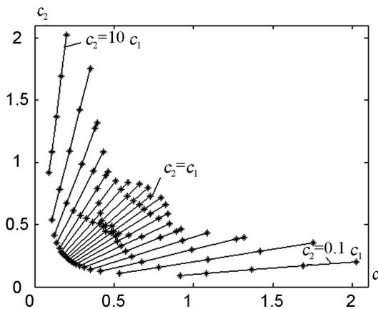
**Figure 6.** The bifurcation points in the plane  $(c_1, c_2)$  for hexagonal array.
