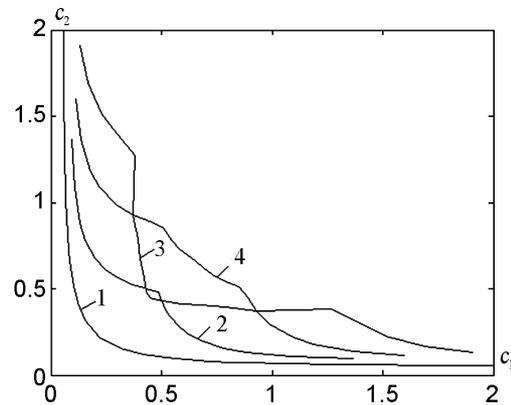
**Figure 7.** The bifurcation lines in the plane  $(c_1, c_2)$  for hexagonal array.
