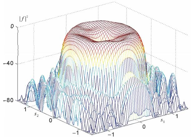
**Figure 24.** The synthesized power DP  $|f|^2$  for the prescribed DP (29) at  $c_1 = 2.0$ ,  $c_2 = 2.236$ .
