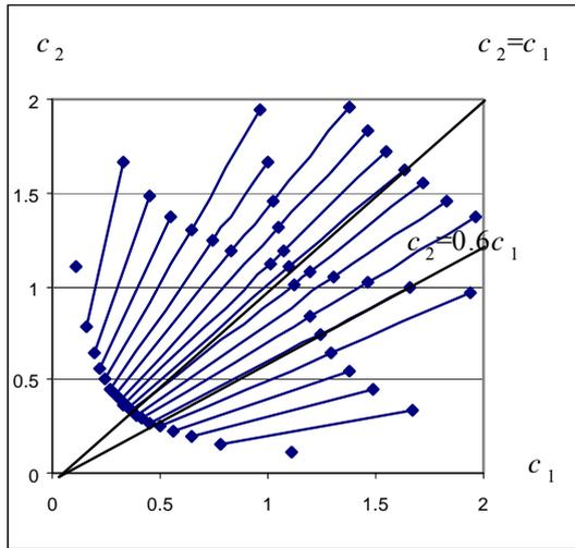
**Figure 2.** The bifurcation points on the beams  $c_2 = \beta c_1$  for plane aperture.
