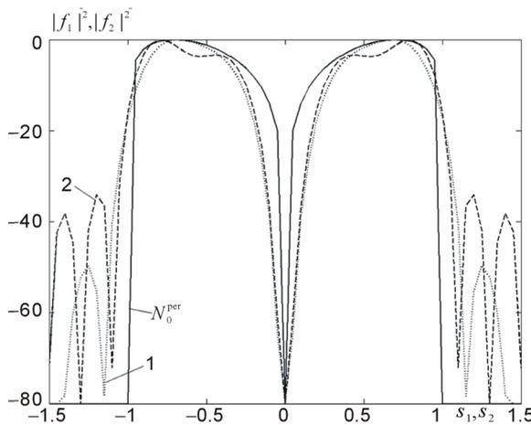
Figure 26. Cross-section of the synthesized DP  $|f|^2$  in the planes  $s_1 = 0$  and  $s_2 = 0$  for the prescribed DP (29).
