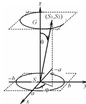
**Figure 1.** Geometry of synthesis problem for plane aperture.
