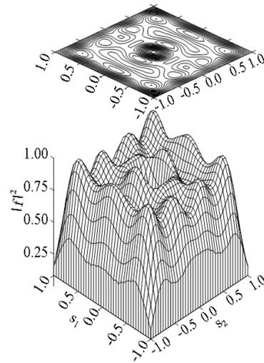
Figure 19. The synthesized power DP  $|f|^2$  corresponding to solution of type 2).
