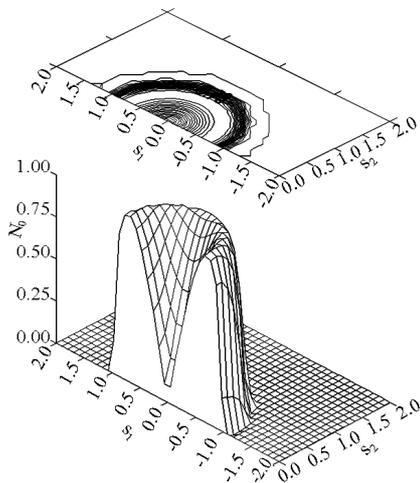
Figure 12. The prescribed power DP (29) in form of the figure of revolution.
