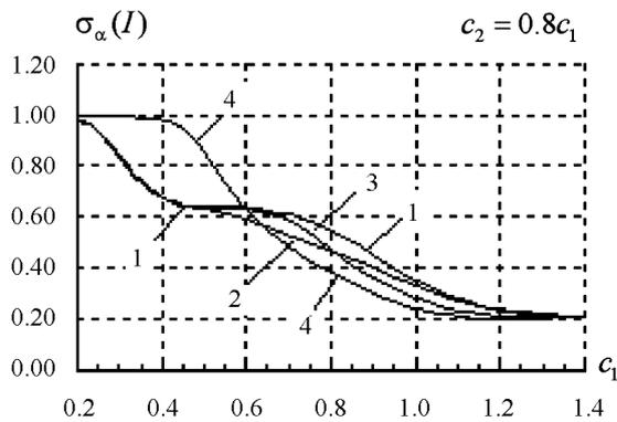
**Figure 22.** The value of functional  $\sigma_\alpha$  for different types of solution to Equation (11) for prescribed power DP (30).
