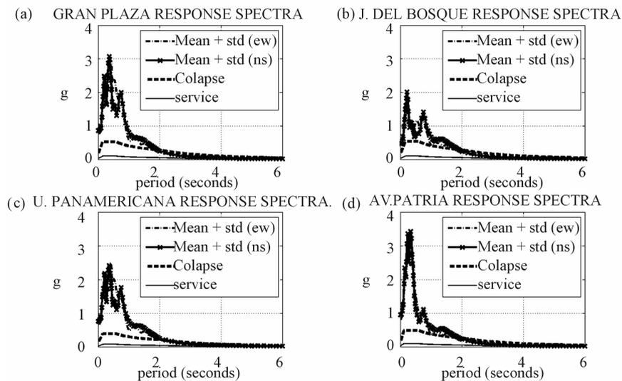
**Figure 10.** Response spectra calculated according to MOC-2008 procedure vs response spectra using seismic records. The different curves represent mean plus standard deviation response spectra for both components, response for a rock site, for edge state of service and for collapse. (a) Gran Plaza site; (b) Eulogio Parra site; (c) Av. Patria site; (d) U. Panamericana site.
