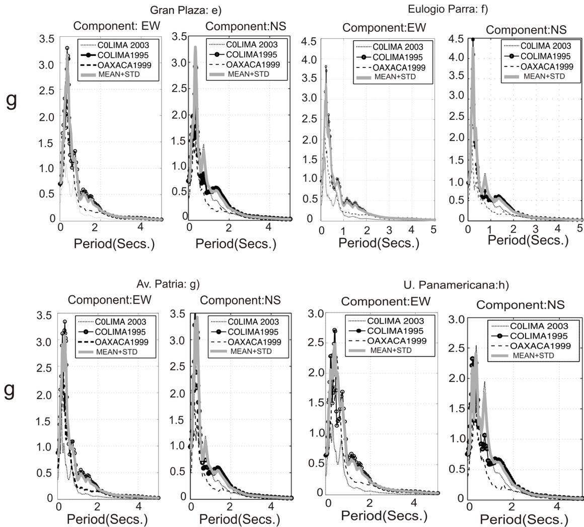
**Figure 8. Response spectra for 5% damping for the eight sites using real records propagating through a layered media. Continuous line represents spectra using the Colima 2003 record, continuous line with dots, the spectra using Colima 1995 record, dotted line represents spectra from the Oaxaca 1999 record. Green line is the mean plus standard deviation. (e) Gran Plaza site; (f) Eulogio Parra site; (g) Av. Patria, site; (h) U. Panamericana site.**
