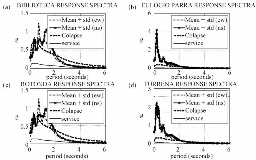
**Figure 9.** Response spectra calculated according to MOC-2008 procedure vs response spectra using seismic records. The different curves represent mean plus standard deviation response spectra for both components, response for a rock site, for edge state of service and for collapse. (a) Biblioteca site; (b) Rotonda site, (c) J. del bosque site; (d) Torrena site.
