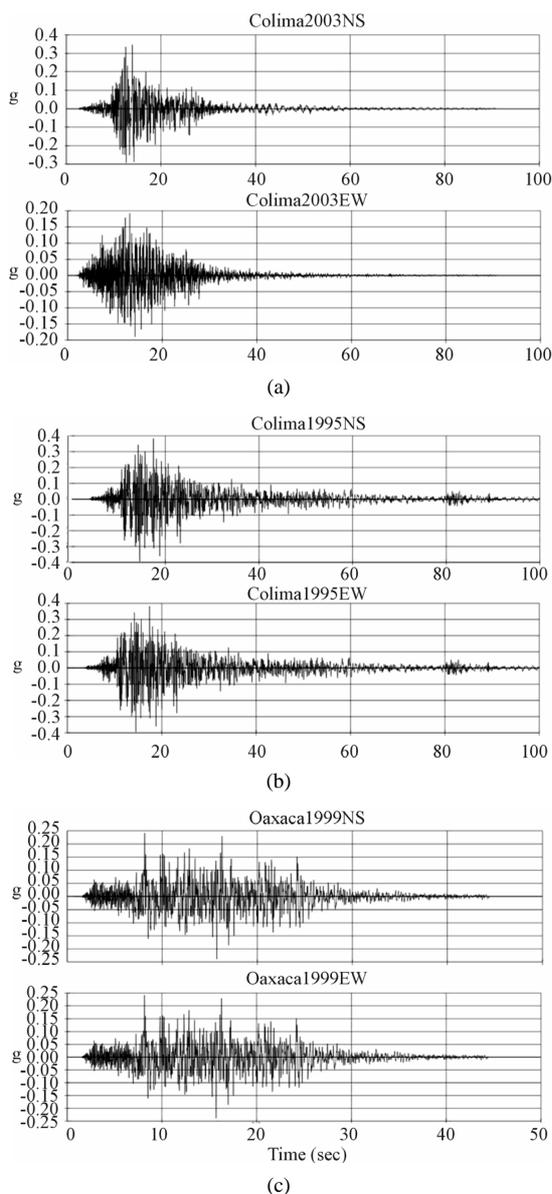
**Figure 3. Horizontal acceleration records used. (a) Colima 2003 (Mw 7.5), (b) Colima 1995 (Mw 7.5), (c) Oaxaca 1999 (Mw 7.5).**
