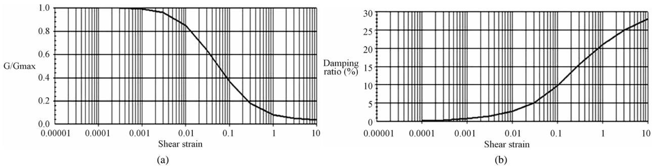
Figure 6. (a) Shear modulus vs shear-strain; (b) Damping ratio vs shear-strain [7,8].
