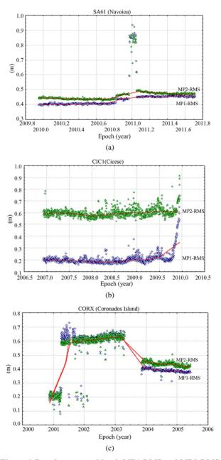
Figure 6. Pseudorange multipath MP1-RMS and MP2-RMS variations, most affected sites: (a) Navojoa (SA61), SNG network; (b) Cicese (CIC1), SCIGN network and Coronados Island (CORX), SCIGN network.
