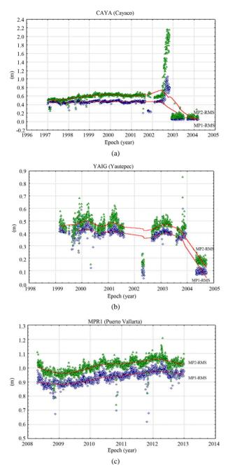
Figure 10. Pseudorange multipath (MP1-RMS and MP2-RMS) variations, most affected sites: (a) Cayaco (CAYA) and Yautepec (YAIG), UNAM network and (c) Puerto Vallarta (MPR1), CORS network.
