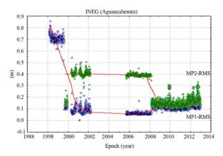
Figure 3. Pseudorange multipath (MP1-RMS and MP2-RMS) variations at site INEG, RGNA network.
