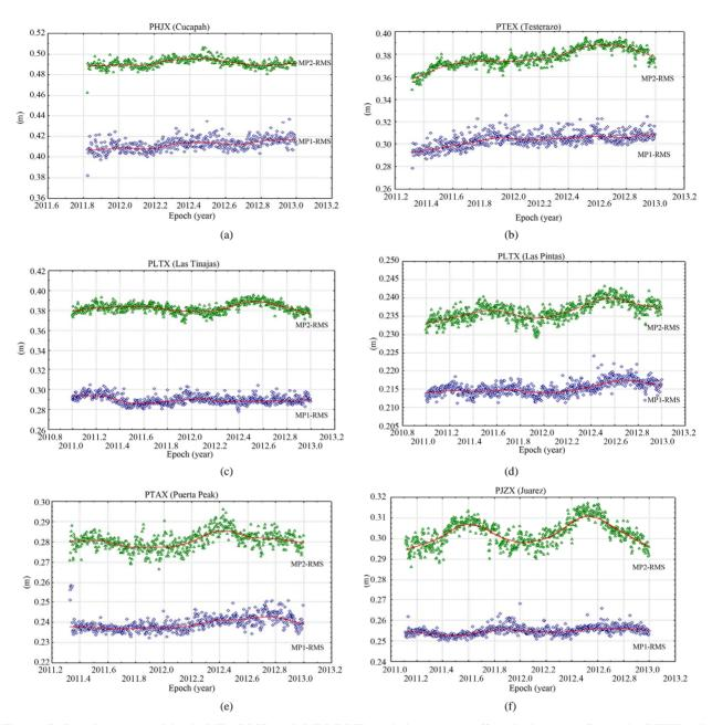
Figure 7. Pseudorange multipath MP1-RMS and MP2-RMS variations, most affected sites: (a) Cucapah (PHJX); (b) Testerazo (PTEX); (c) Las Tinajas (PLTX) and least affected sites: (d) Las Pintas (PLPX); (e) Puerta Peak (PTAX); (f) Sr. Juárez (PJZX), PBO network.
