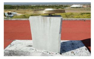
Figure 2. Aguascalientes (INEG) station with choke-ring antenna, RGNA network. Date of photo February, 2000.
