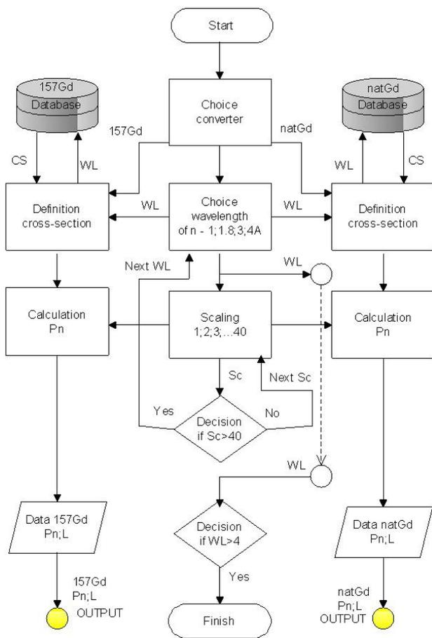
**Figure 2.** Calculation algorithm diagram of absorption path of neutrons in substance.
