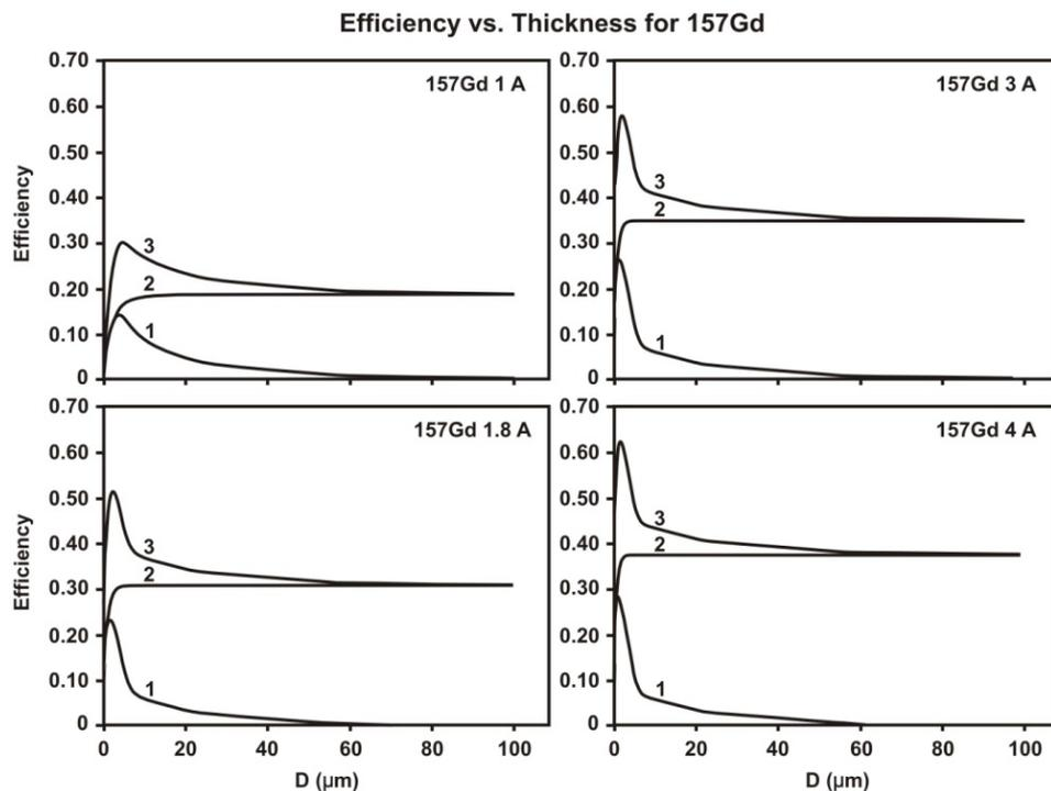
Figure 11. Dependence of the neutron registration efficiency of the  $^{157}$  isotope of Gadolinium converter on its thickness. Curves 1 and 2 correspond to emission of electrons into the front and back hemisphere, respectively, curve 3 is their sum.
