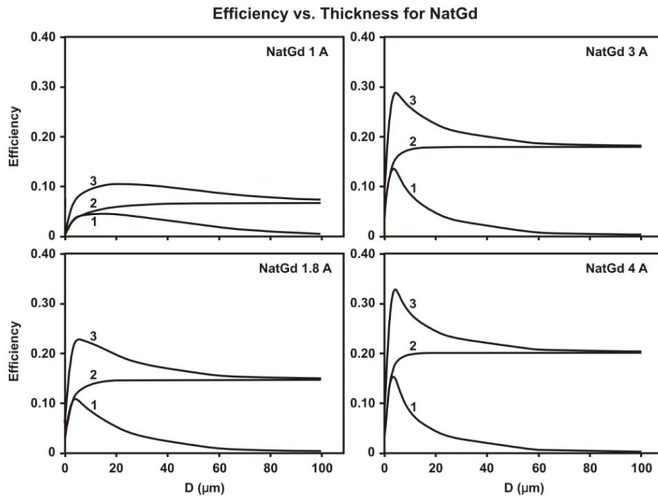
Figure 10. Dependence of the neutron registration efficiency of the natural Gadolinium converter on its thickness. Curves 1 and 2 correspond to emission of electrons into the front and back hemisphere, respectively, curve 3 is their sum.
