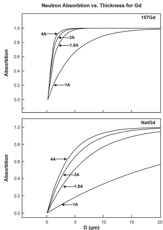
**Figure 3.** Curve absorption path of neutrons for lengths of waves 1, 1.8, 3 and 4 Å for natural Gadolinium and it 157 isotopes (output data).
