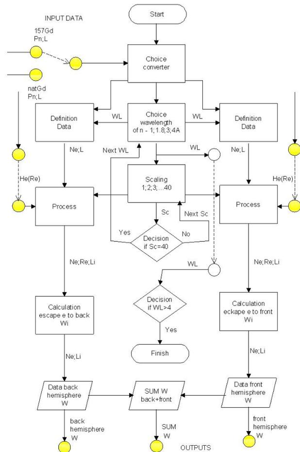
Figure 9. Scheme algorithm calculation of the efficiency of converters.
