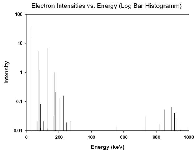
**Figure 6. Intensity of internal conversion electrons emitted in the reaction  $^{157}\text{Gd} (n, \gamma) ^{158}\text{Gd}$  depending on their energy by 100 neutrons (output data).**
