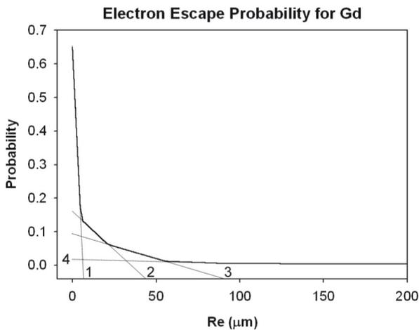
Figure 8. Probability of exit of isotropic emitting secondary electrons from Gadolinium foils of various thicknesses, in view of their intensity (output data).
