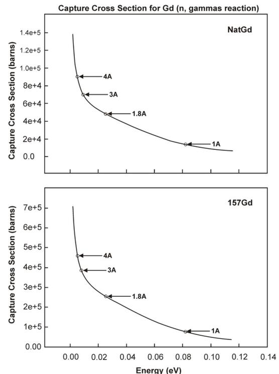
**Figure 1.** Cross-section of thermal neutrons capture, for the reaction ( $n, \gamma$ ), depending on energy of neutrons for natural Gadolinium and its 157 isotope (input date).
