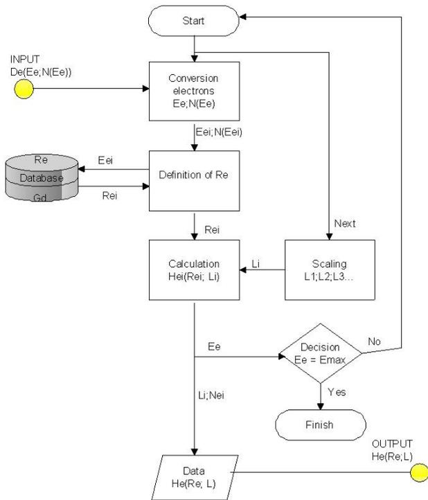
Figure 7. Scheme of algorithm calculation of ability an electrons exit from the converter body.
