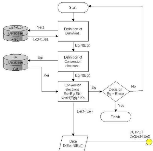
**Figure 5. Diagram of algorithms for calculation of internal conversion electrons.**
