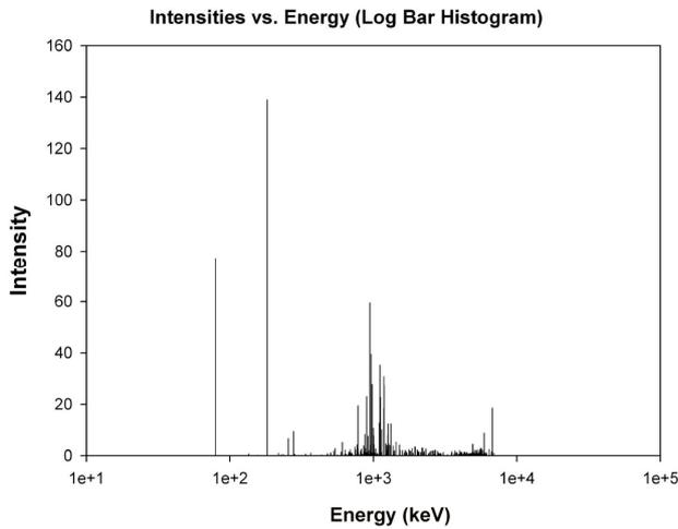
**Figure 4. Histogram of dependence of intensity of gamma-quanta with energy for the reaction of  $^{157}\text{Gd} (n, \gamma) ^{158}\text{Gd}$  by 100 neutrons (input data).**
