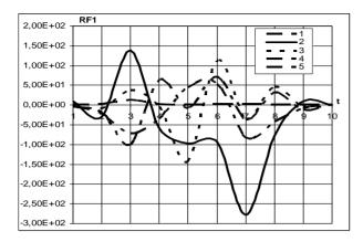
Figure 1. The change of the tangential component of the Lorentz force  $\rho F_{\zeta}^{\wedge}$  depending on the time when s = 0.05 m all options for changing the external electric current  $J_{\theta CT}$ :
