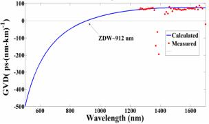
Figure 3. Calculated dispersion profiles of seven-core fiber as well as the measurements.
