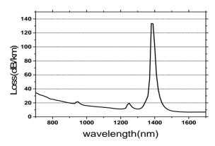
Figure 4. The attenuation spectrum of seven-core PCF.
