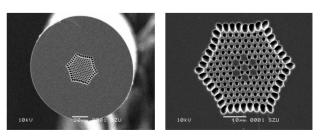
Figure 1. SEM pictures of seven-core PCF: (a) the end face (b) the core region.
